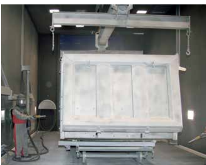
Blast room with work piece lifting device for trailers
