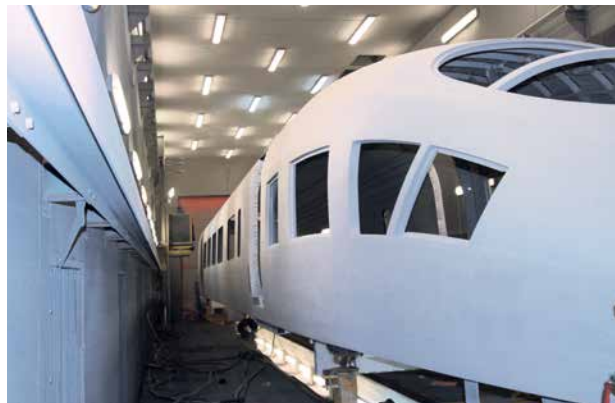
Blast room for rail vehicles with lifting platforms
