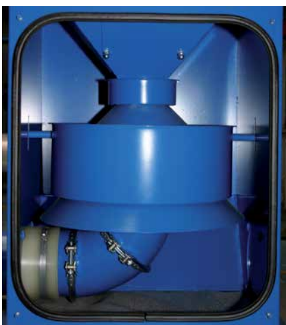
Schematic view and example of a blast media reconditioning unit with wind sifting
