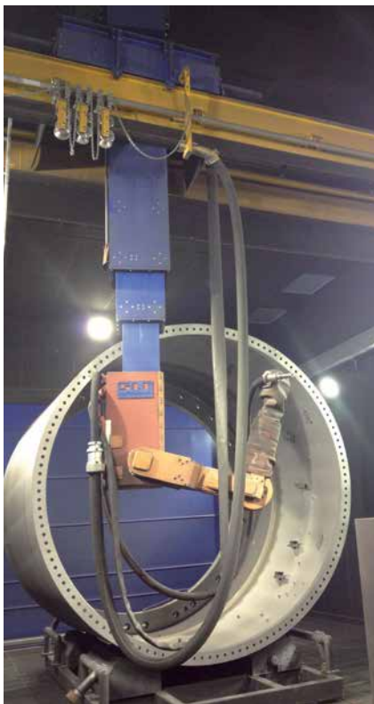
Automatic blasting of towers for wind power plants
