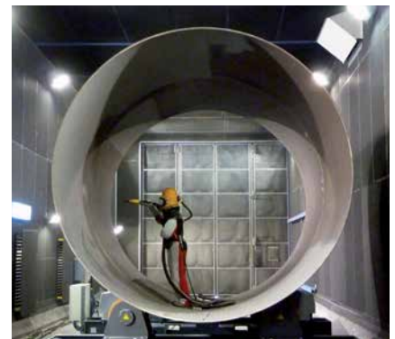
Blast room for components of wind power plants
