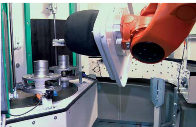
Blast cleaning system for planetary carriers with automatic loading and unloading device
