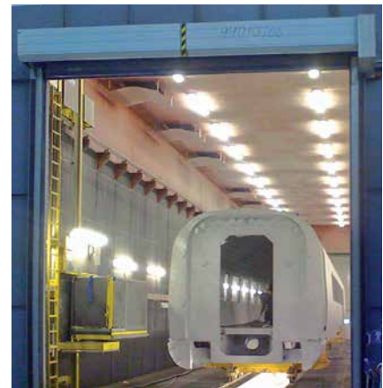
Blast room for blasting of rail vehicles with swivelling platforms
