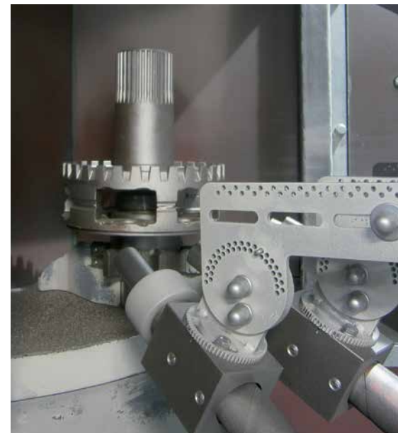
Shot peening system for planetary carriers with automatic work piece handling
