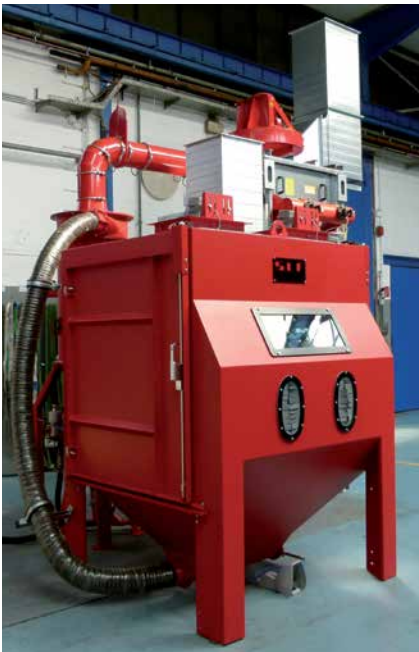
Hand blast cabinet with pneumatic blast media transport
