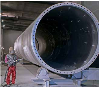
Blast room with work piece rotating device for wind tower segments
