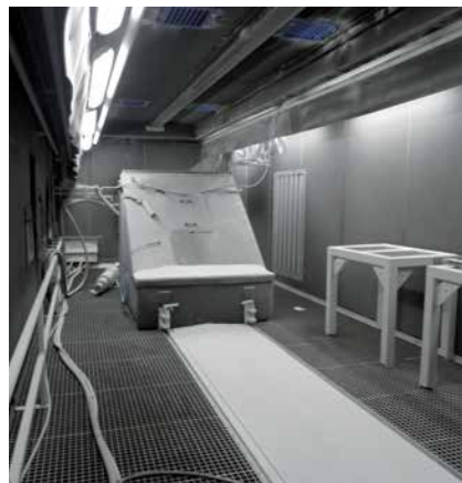
Blasting machine with automatic work piece rotating device and nozzle oscillation for blasting of rolls
